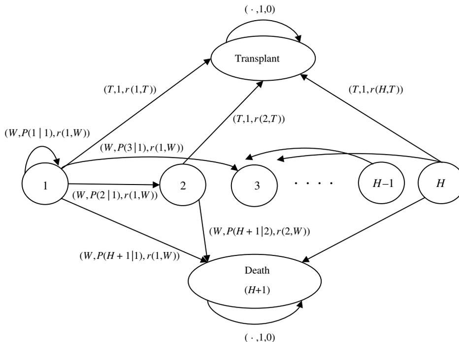
Note. The labels (*a*(*h*),  $P(j | h)$ , *r*(*h*, *a*)) on each arc represent the action taken at state *h*, the probability that the patient will move to state *j* when her current state is *h*, and the reward obtained by taking action *a* in health state *h*, respectively. Note that this figure does not show all possible transitions.
