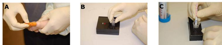
Figure 3. Illustration of future assay concept. Blood is collected from the heel stick of an infant (A), processed in a portable heater device (B) and assayed with the carbon p24 rapid assay (C).
