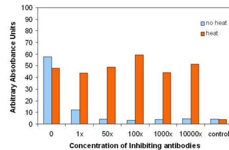
Figure 2. Assay results of 1ng/mL p24 antigen in the presence of increasing concentrations of competing anti-p24 monoclonal antibodies.
